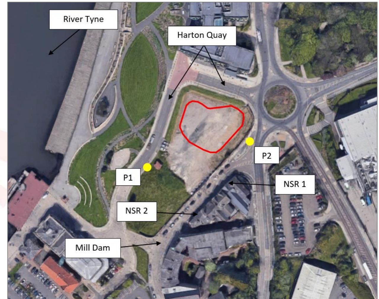
Figure 1: Proposed site outlined in red, measurement positions indicated in yellow, and NSR identified
