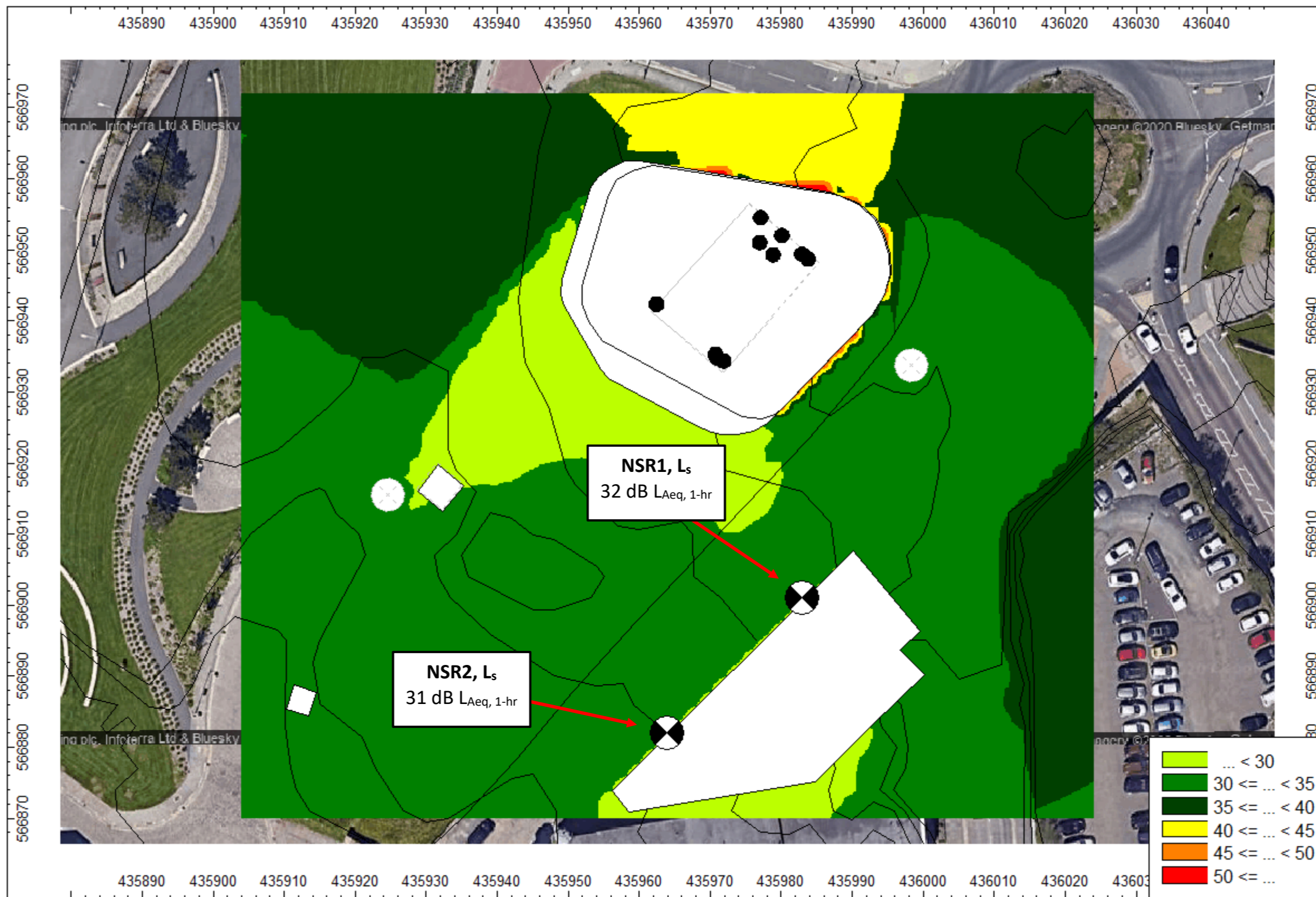
Figure 3: Sound contours at 11 m, showing the calculated specific sound level, L Aeq, 1 hr based on current proposals
